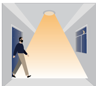
After power on,when motion detected,light ON.
