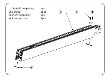
loose the 2 screws at the lamp end, and pull out the inner connector from the lamp body, then fix the inner connector by 2 screws again, insert the inner end caps at both sides.
