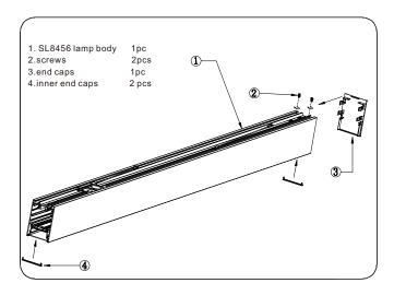
Just fix the end cap at the last end by screws, and insert the two inner end caps.
