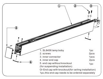
Firstly, loose the 2 screws at the lamp end, and pull out the inner connector from the lamp body, then fix the inner connector by 2 screws again. After finishing the wiring connection(see the steps on the continuous connection), fix the end cap by screws and insert the inner end caps at both sides.
