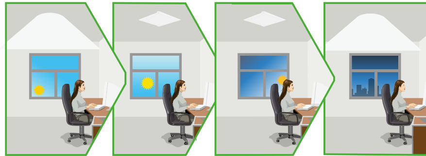
The light turns on at full or dims to maintain the lux level. The light output regulates according to the level of natural light available.
