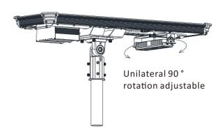
4. Adjust the vertical angle of the light-emitting module;
