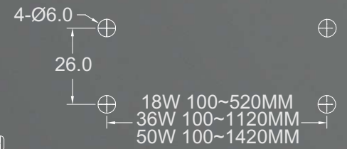
Drill hole size of ceiling installation
