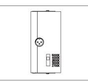
Turn the dip switch to the desired color temperature level.
