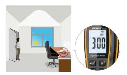
2) Take a lux meter and place it on the desktop or workbench to observe whether the current brightness of the lamp meets customer's needs. If not, 50%-100% lux can be set in the "TASK LIGHT LEVEL" button until it meets the customer's requirements
