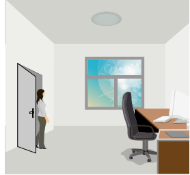
With sufficient natural light, the light does not switch on when presence is detected.
