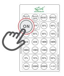
3) After brightness setting, click "ON" in the DAYLIGHT HARVESTING function key to open this function. The sensor will automatically recognize the lux of the current desktop or workbench, and the function setting is completed.
