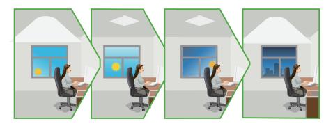
The light turns on at full or dims to maintain the lux level. The light output regulates according to the level of natural light available.
