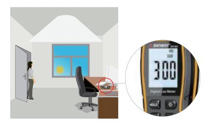
2) Take a lux meter and place it on the desktop or workbench to observe whether the current brightness of the lamp meets customer's needs. If not, 50%-100% lux can be set in the "TASK LIGHT LEVEL" button until it meets the customer's requirements
