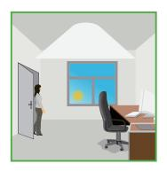
The light will always switch ON automatically on detecting presence or manually with power switch (even without detecting presence) - When DAYLIGHT HARVESTING is enabled, the light output regulates between Task and Stand By levels according to the level of natural light available.
