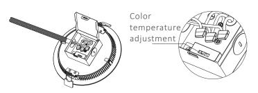
3. Connecting the cables with wire nuts, then toggle the switch in the J-box to select the correct color temperature
