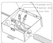
9. Insert the junction box through the hole in the ceiling.
