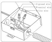
9. Insert the junction box through the hole in the ceiling.
