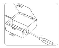
8.Connect the junction box to the slim down light, tighten the connectors by hand. The slot of the male/female connectors need to aligned before inserted.
