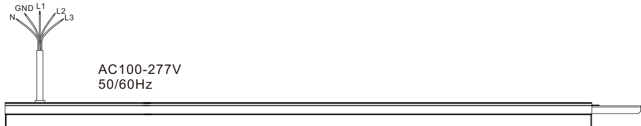
SL5550 non-dimming AC connection diagram
