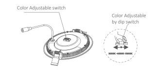
4. Blue wire is connected to N; Brown wire is connected to L; and yellow-green wire is connected to G.
