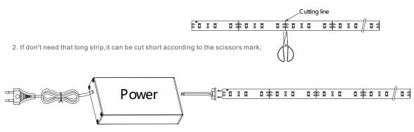
3. The cut strips can be connected via accessories connectors, then the strips are connected to power supply.
