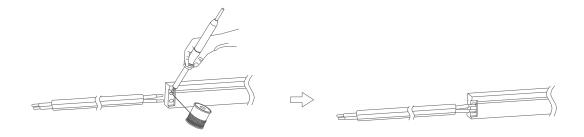
5. Put the plug on the line and repeat the gluing steps as shown in Figure 2. Then plug the lamp strip into the plug and complete the installation, as figure 5.
