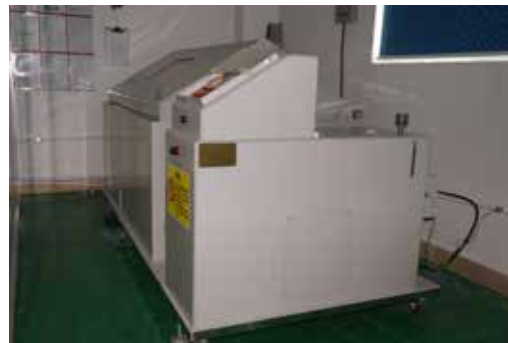
▲ Salt spray test
