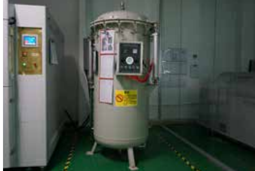
▲ IP rating test
